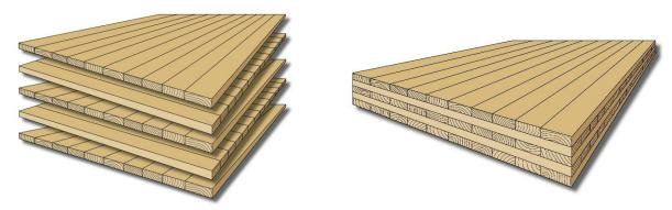
Figure 1. CLT layers shown separated (left) to illustrate alternating intermediate layers oriented perpendicular to the long direction of the CLT panel. Figure at right shows CLT in its final solid configuration.
