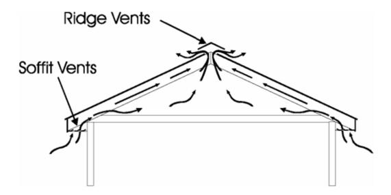
Figure 1. Illustration of attic ventilation with air flowing in through soffit vents and out through ridge vents.
